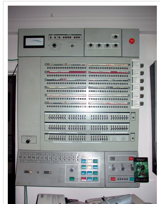
System/360 (Model 65) operator's console, with register value lamps and toggle switches and buttons (middle of picture) .
