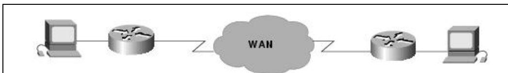
Figure: A Typical Point-to-Point Link Operates Through a WAN to a Remote Network
