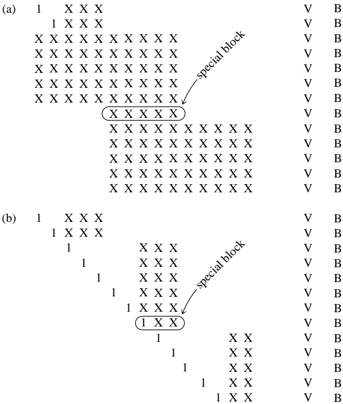
Figure 17.6.1. FDE matrix structure with an internal boundary condition. The internal condition introduces a special block. (a) Original form, compare with Figure 17.3.1; (b) final form, compare with Figure 17.3.2.
