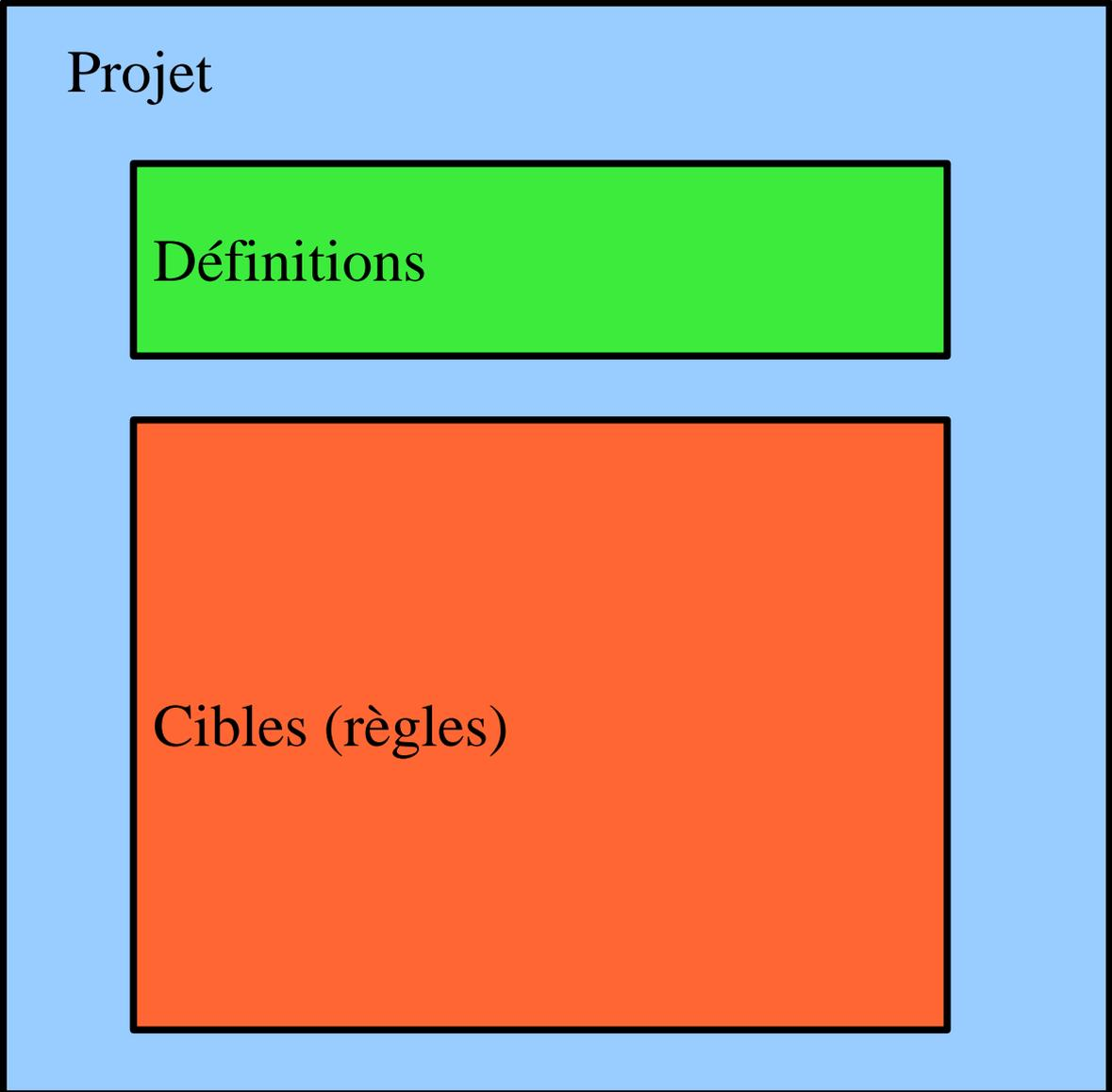
A diagram illustrating the structure of an Ant build.xml file. It consists of a large light blue rectangle representing the 'Projet' (Project) element. Inside this rectangle, there are two smaller rectangles stacked vertically. The top one is green and labeled 'Définitions' (Definitions). The bottom one is orange and labeled 'Cibles (règles)' (Targets (rules)).
